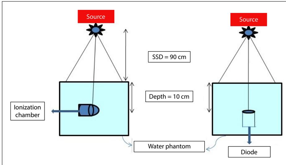
**Figure 1.** Detectors position in the central axis of the beam. SSD — source to surface distance
