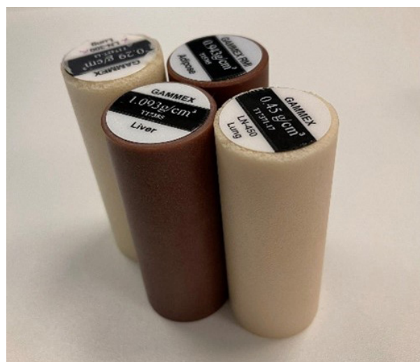
Figure 4. A customized rod that could be equipped with cylinders of different densities was connected to the actuator as a lung insert in the study
