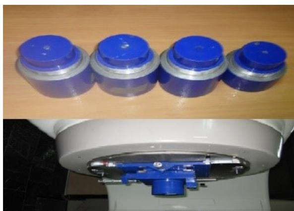
**Figure 2.** A photograph of four conical collimators and a collimator holder used in the present work
