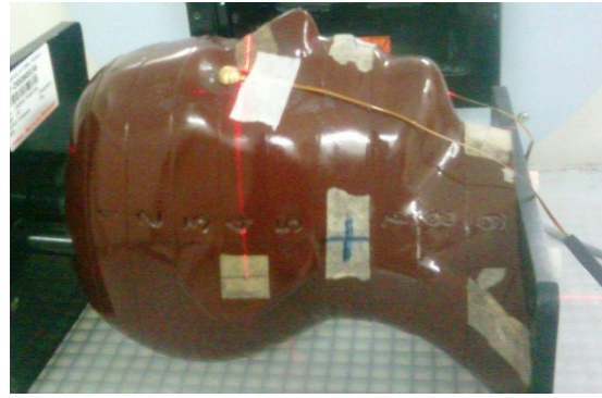
Figure 4. Position of standard sensitivity MOSFET dosimeter with buildup cap on the eye level in Rando phantom
