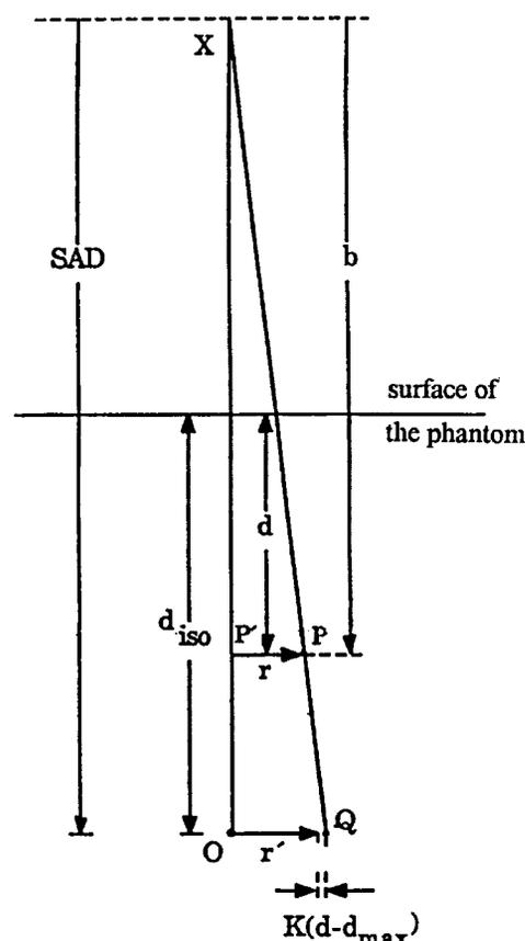
Fig. 1. Conceptual diagramme showing dose calculation for a single beam as part of stereotactic multiple-arc therapy. The dose is calculated at point P. The x-ray source is at X and the isocentre is at O. All other quantities are defined in the text (Luxton et al., 1991).
