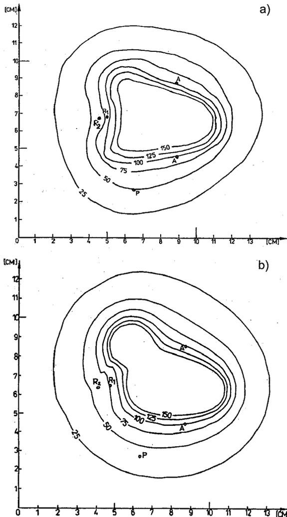
Dose distribution in XY plane: (a) from a stationary unit, (b) from a mobile unit.
