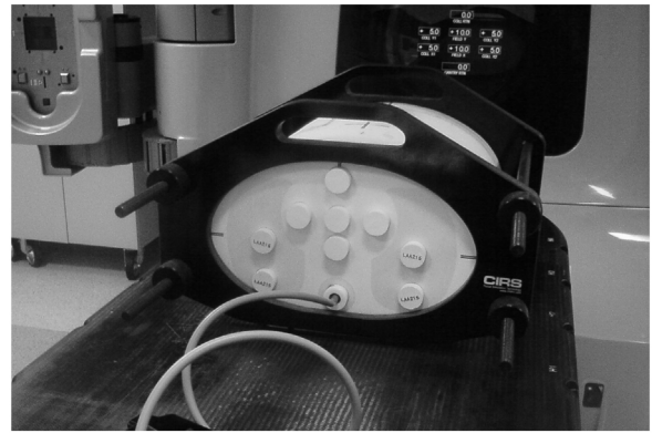
Fig. 2. CIRS IMRT thorax phantom – model 002LFC used for on-site audits of 3D conformal teleradiotherapy techniques.gr2
