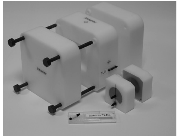
Fig. 4. The phantom used for auditing with an encapsulated adaptor (aside) for films and TLD capsules [2].gr4
