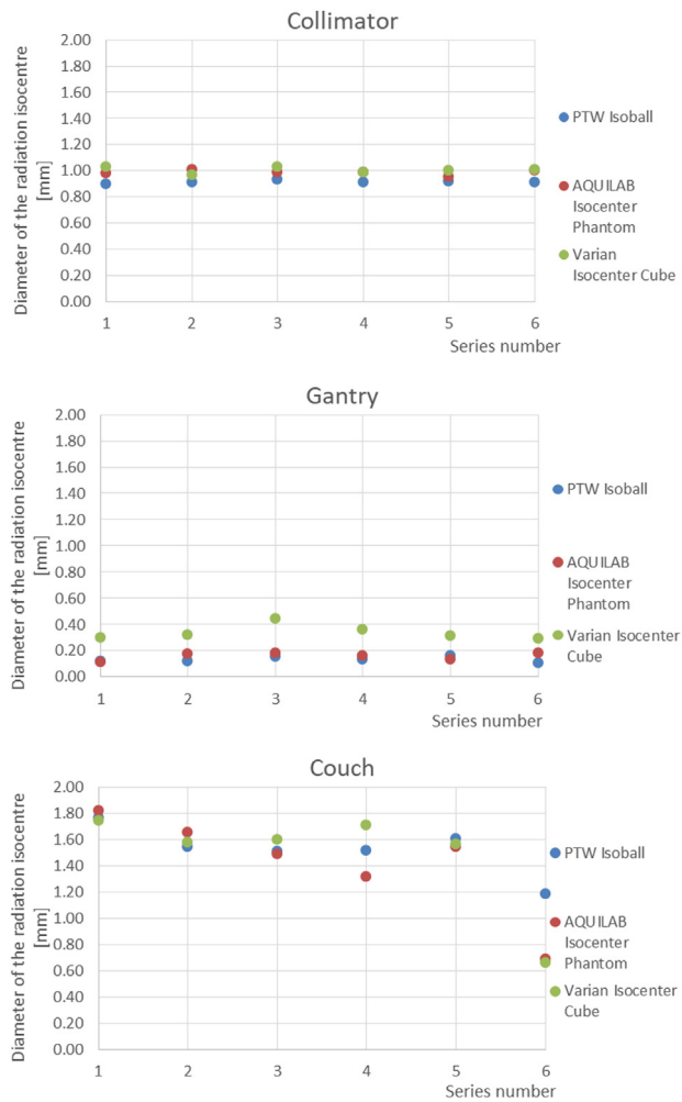
Fig. 3. Diameter of the radiation isocentre for TrueBeam with aS1000 EPID, for: a) collimator, b) gantry, c) couch.
