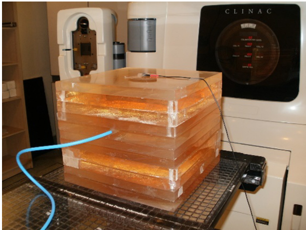
Fig. 2 – The setup used for the measurements of solid-state detector calibration factor as a function of radiation field size.
