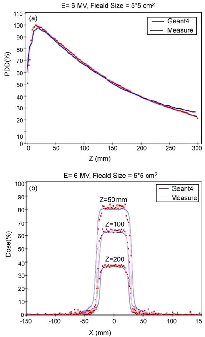
**Fig. 2 – (a) Depth-dose profile. (b) Lateral dose profiles at 50, 100, and 200 mm depth for the 5 cm × 5 cm field, with the 6-MV beam. The blue lines refer to measured data; red dots refer to Geant4 Monte Carlo results.**
