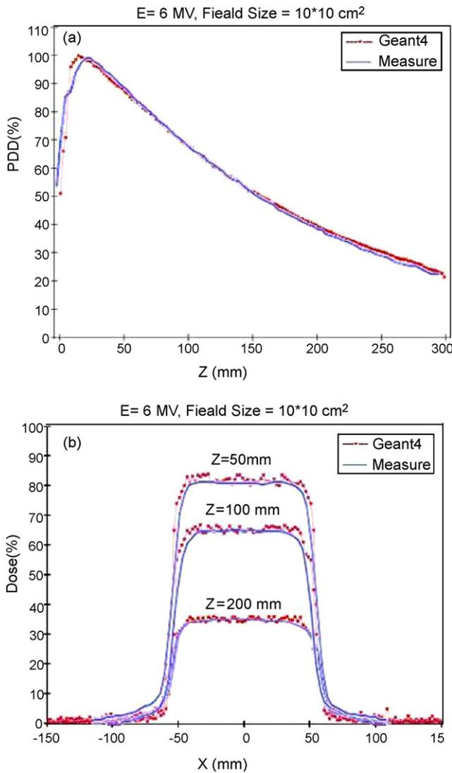
**Fig. 3 – (a) Depth-dose profile. (b) Lateral dose profiles at 50, 100, and 200 mm depth for 10 cm × 10 cm field with a 6-MV beam. The blue lines refer to measured data, and red dots refer to Geant4 Monte Carlo results.**
