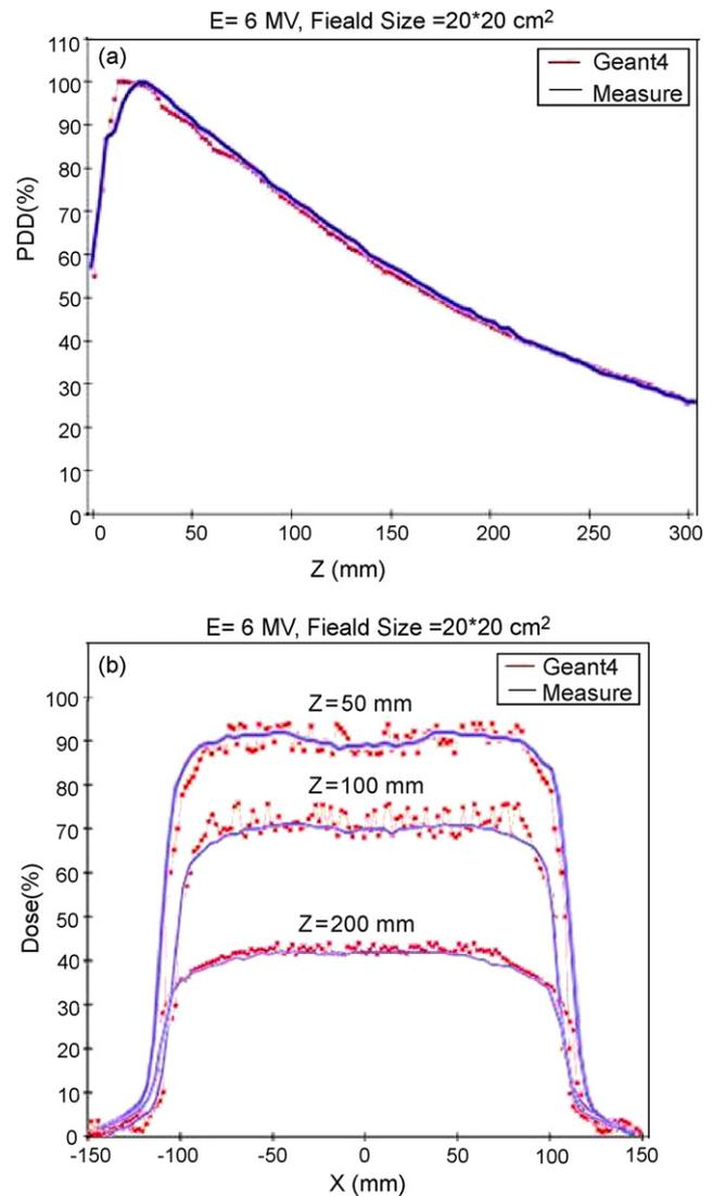
**Fig. 4 – (a) Depth-dose profile. (b) Lateral dose profiles at 50, 100, and 200 mm depth for 20 cm × 20 cm field, with 6-MV beam. The blue lines refer to measured data, red dots refer to Geant4 Monte Carlo results.**
