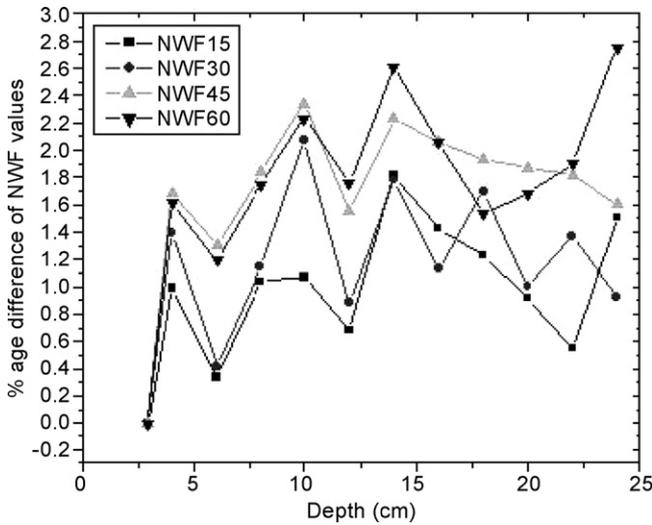
**Fig. 5 – Percentage difference of the experimental and TPP (V 3.8) calculated values without incorporating  $C_{hard}$ ,  $a_1$  and  $a_2$  as a function of depth keeping the field size constant (10 cm × 10 cm) for a 15 MV beam.**
