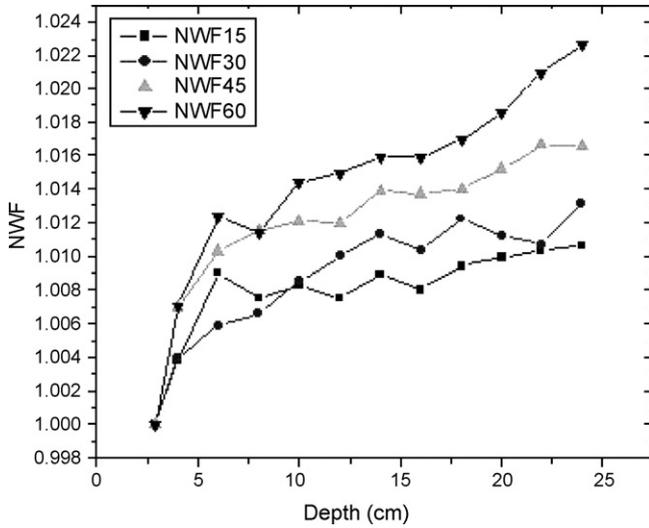
**Fig. 1 – Experimentally observed normalized wedge factor (NWF) as a function of depth for a fixed field size (10 cm × 10 cm) for 15 MV photon beam.**
