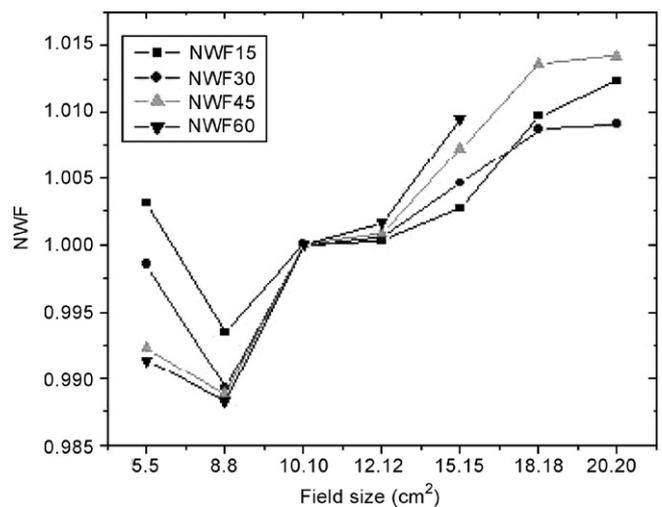
**Fig. 8 – NWF as a function of field size keeping the depth constant (10 cm) for a 15 MV photon beam. TPP (V 3.8) was modified by incorporating the values of  $C_{hard}$ ,  $a_1$  and  $a_2$  in it.**
