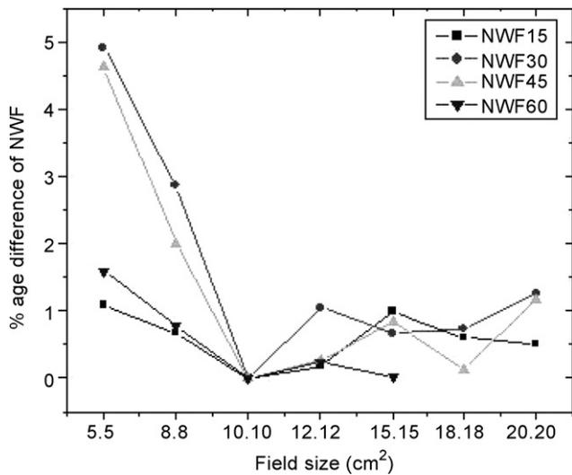
**Fig. 6 – Percentage difference between experimental and TPP (V 3.8) calculated NWF values without using  $C_{hard}$ ,  $a_1$  and  $a_2$  as a function of field size keeping the depth constant (10 cm) for a 15 MV beam.**
