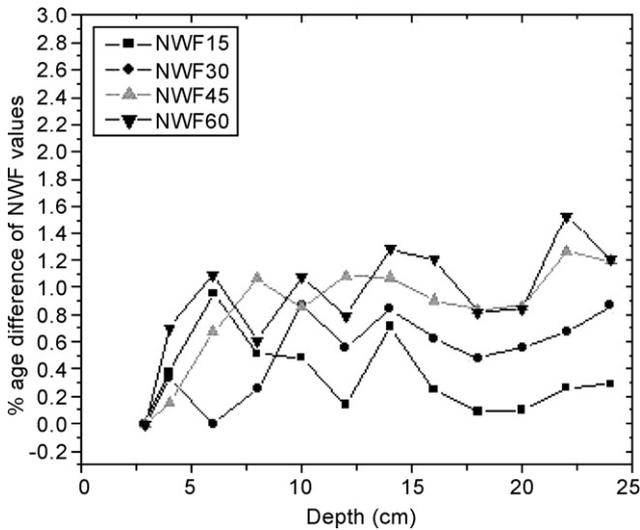
**Fig. 9 – Percentage difference of the experimental and TPP (V 3.8) calculated NWF values incorporating the values of  $C_{hard}$ ,  $a_1$  and  $a_2$  as a function of measurement depth keeping the field size constant (10 cm × 10 cm) for a 15 MV beam.**
