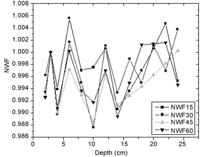
**Fig. 3 – Calculated NWF as a function of depth keeping the field size constant (10 cm × 10 cm) for 15 MV photon beam using TPP (V 3.8) without incorporating  $C_{hard}$ ,  $a_1$  and  $a_2$ .**
