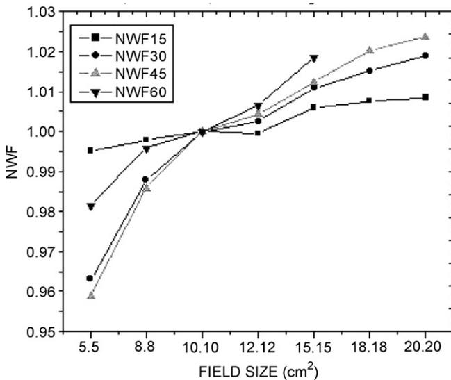
**Fig. 2 – Experimentally observed normalized wedge factor (NWF) as a function of field size for a fixed depth (10 cm) for 15 MV photon beam.**
