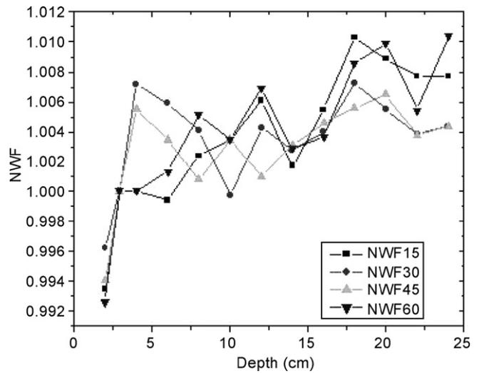
**Fig. 7 – TPP (V 3.8) calculated NWF values as a function of depth keeping the field size constant (10 cm × 10 cm) using  $C_{hard}$ ,  $a_1$  and  $a_2$  values for a 15 MV photon beam.**
