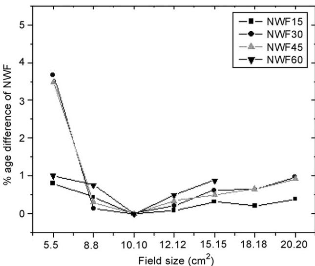
**Fig. 10 – Percentage difference among the experimental and modified TPP (V 3.8) calculated NWF values as a function of field size keeping the measurement depth constant (i.e. 10 cm) for a 15 MV beam.**
