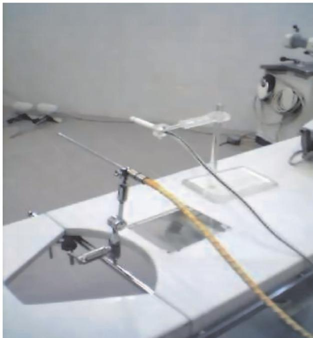
**Fig. 2.** Measurement setup shows the applicator and Farmer type  $0.65 \text{ cm}^3$  ionization chamber.
