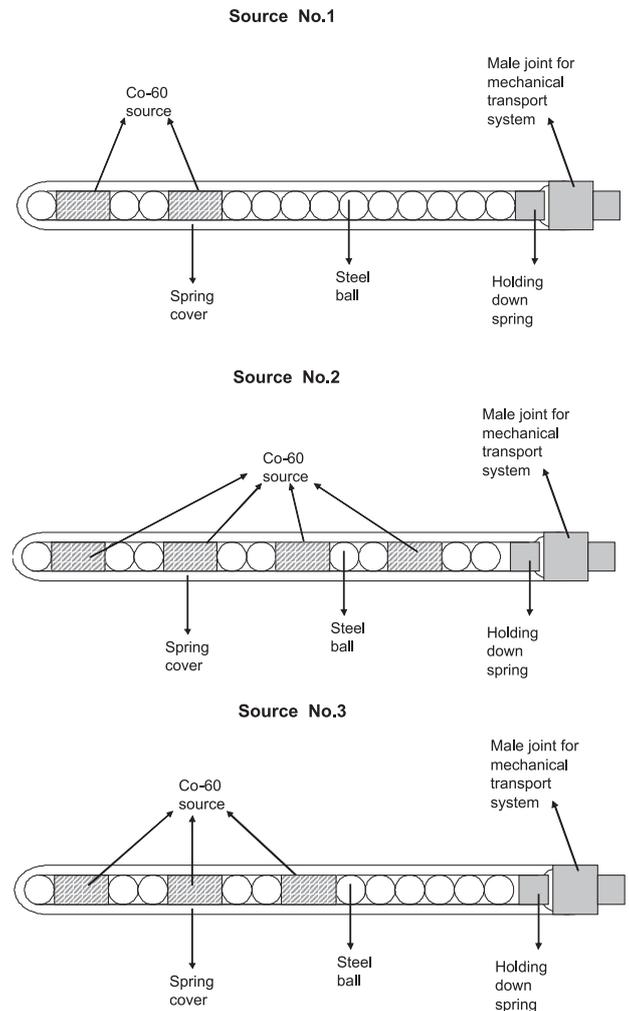
**Fig. 1.** Schematic diagrams of GZP6  $^{60}\text{Co}$  braid type sources used for intracavitary treatments.
