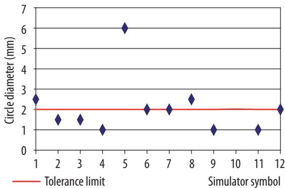
**Figure 5.** Agreement of the couch column rotation axis with collimator rotation axis.
