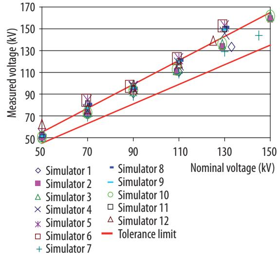
**Figure 6.** Agreement between measured high voltage values with console settings.
