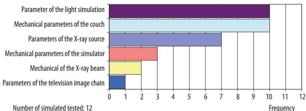
Figure 8. Frequency of tolerance limit violations for particular groups of parameters.
