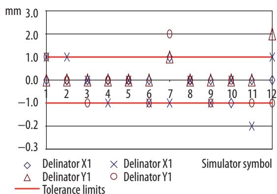
**Figure 4.** Accuracy of the delineator positions in relation to the reference field (5x5cm).
