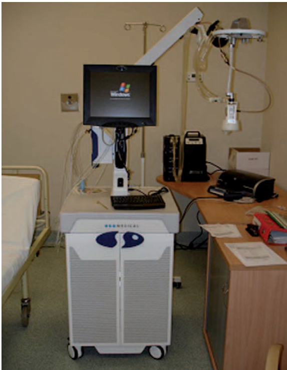
Figure 3. An example of equipment for superficial and interstitial hyperthermia (BSD 500 hyperthermia system) operating on microwaves of 915MHz.
