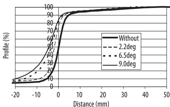
**Figure 3.** Profiles for asymmetric open and modified photon field at 2cm depth. Light field edge there is at zero position.
