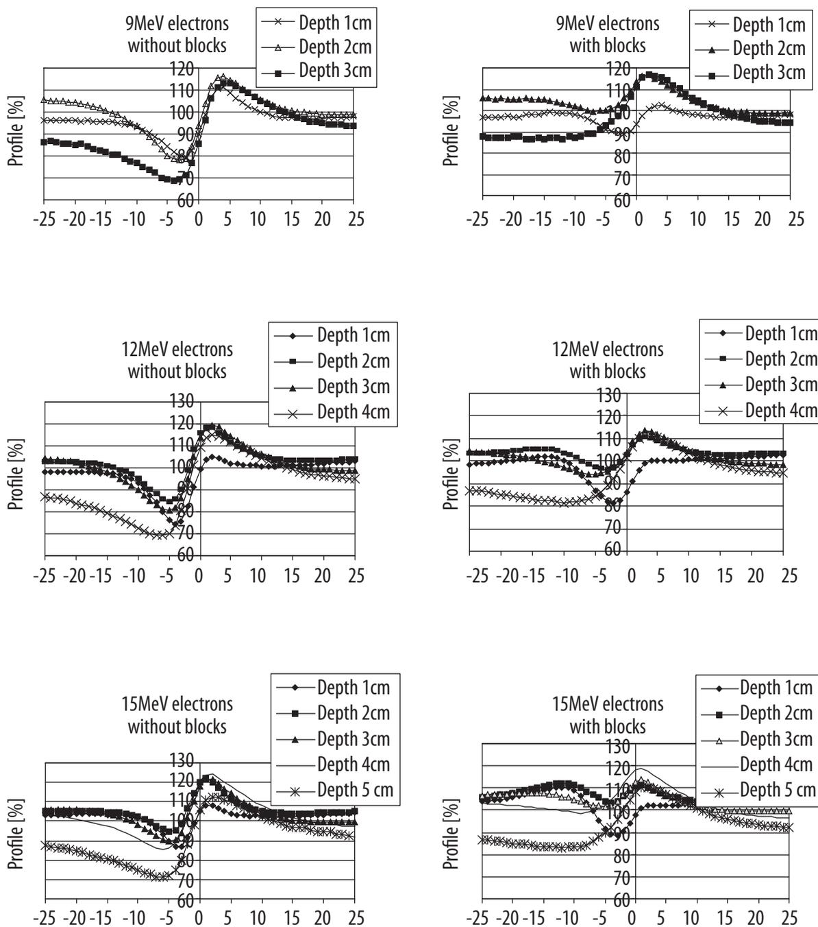
**Figure 4.** Comparison of dose distribution in the matching region for 9, 12 and 15MeV electron beams and 6MV photon beam with and without block. Electron beams are always on the negative side of the axis. easurements.
