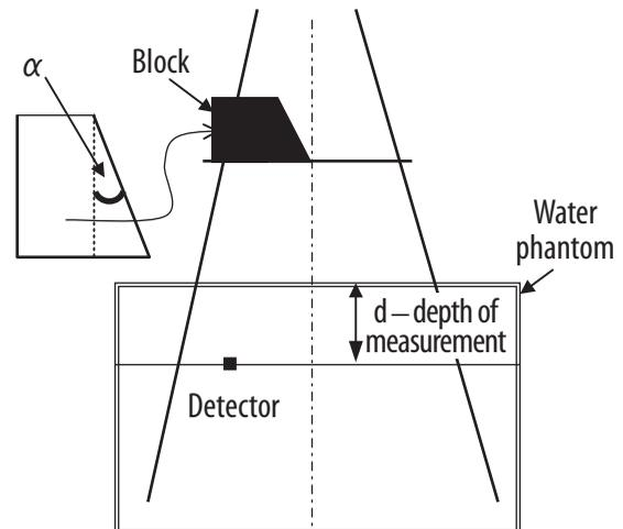
**Figure 2.** Modified block and geometry of measurements.
