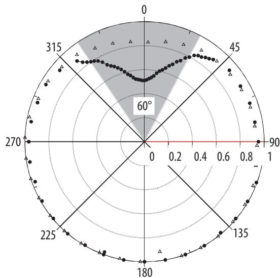
**Figure 2.** Polar plots of dose attenuation effects of the guide wire. Full dots – dose distribution with guide wire present; open triangles – dose distribution without guide wire.
