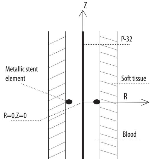
**Figure 4.** The model for stent attenuation by MC calculation.
