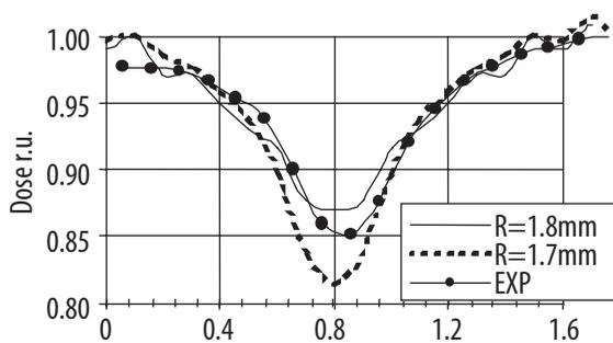
**Figure 3.** Dose distribution (relative units) along a linear source, behind the stent, as measured by the GAF chromic foil – full dots. The calculated distributions for R=1.7mm and 1.8mm were added to show the consistency of measurements with the calculations.
