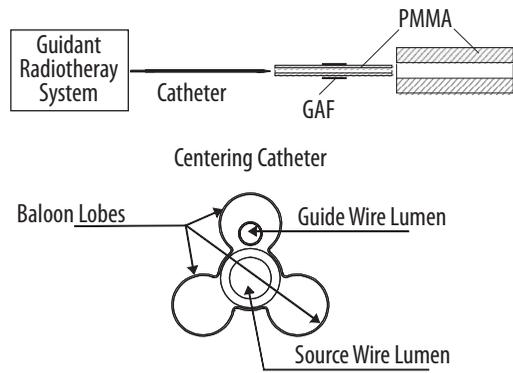
**Figure 1.** Expanded view of measuring set up for studying the shielding effect of the guide wire and the stent struts.
