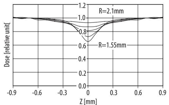
**Figure 5.** Comparison of longitudinal dose distribution at the different distances, R(mm), 1.55, 1.6, 1.7, 1.8 and 2.1 from the axis of the source.
