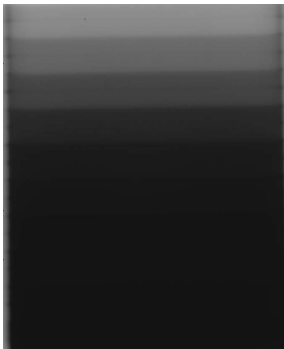
Figure 5. An example image of EDR2 film with 10 discrete OD levels. The film was irradiated using a single X-15MV field of size 15 \times 20 \text{ cm}^2 modulated with a programmed dMLC step wedge.
