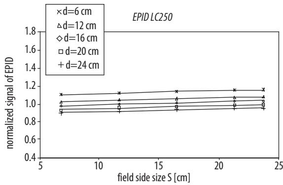
**Figure 4.** EPID signals (PV LC250) as a function of field side size (S) at varying phantom thicknesses (d).
