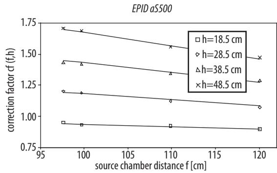
**Figure 3.** The relationship between dose rate measuring by ionization chamber and EPID signal for various distances (f) at the function of (h) –PV aS500.
