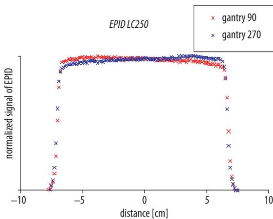
**Figure 6.** Beam profiles of square fields, measured using an EPID 140 cm from the source at 90° and 270° gantry positions of the linear accelerator (PV LC250).
