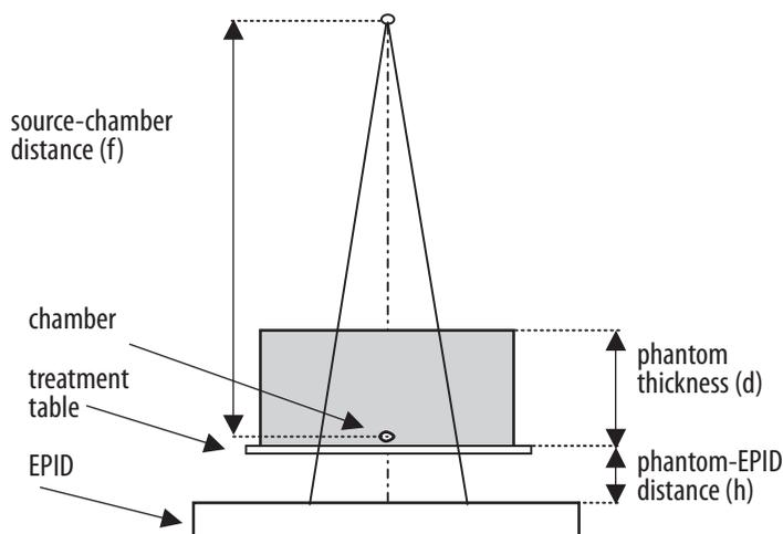
**Figure 1.** A schematic diagram of the experimental set-up for measurements.
