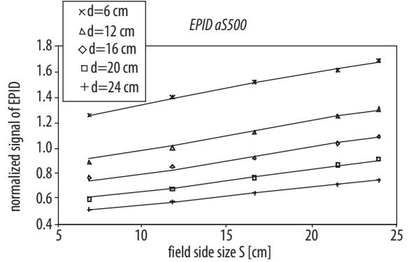
**Figure 5.** EPID signals (PV aS500) as a function of field side size (S) at varying phantom thicknesses (d).
