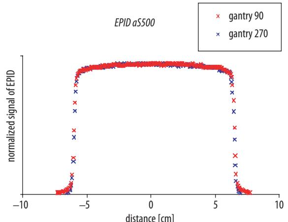
**Figure 7.** Beam profiles of square fields, measured using an EPID 140 cm from the source at 90° and 270° gantry positions of the linear accelerator (PV aS500).
