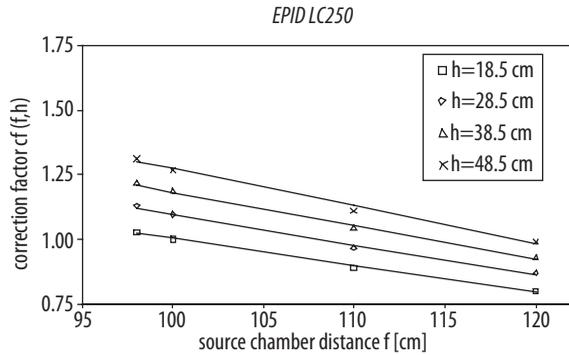
**Figure 2.** The relationship between dose rate measurements by ionization chamber and EPID signal for various distances (f) at the function of (h) – PV LC250.
