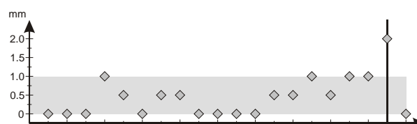
Figure 2a. Laser centration: deviation between the laser beam position and the isocentre (Oldelft).
