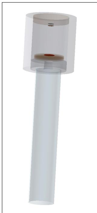
**Figure 3.** Simplified model of the beam forming system used for preliminary design of the primary and secondary scattering foils
