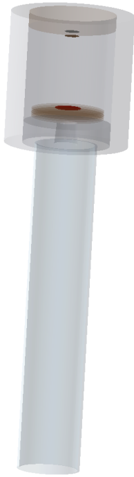
Figure 3. Simplified model of the beam forming system used for preliminary design of the primary and secondary scattering foils
