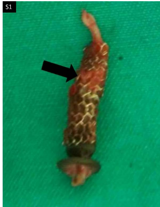
Figure S1. The intraoperative image shows a fractured and excised internal carotid artery stent (arrowhead)
