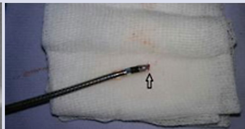
Figure 3. Macroscopic view of the fractured lead
