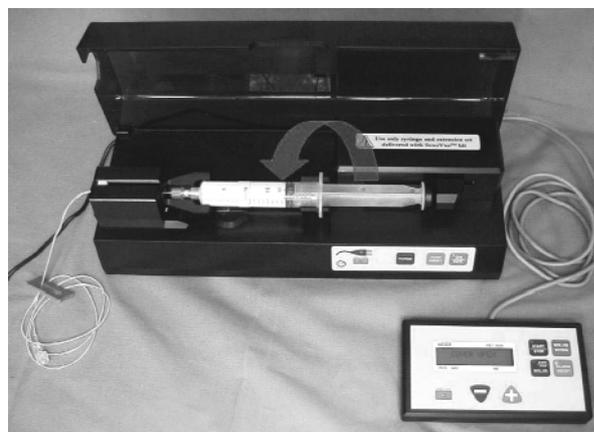
**Figure 1.** Infusion pump BR-INF 100 (Bracco Research, Geneva, Switzerland)
