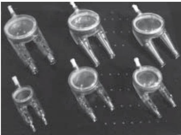
Figure 3. Artificial 10, 25, 30, 50, 60 and 80 mL ventricles available in the Berlin Heart Excor system
