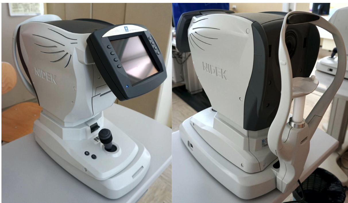
FIGURE 1. Nidek ARK-1 table-mounted refractometer
