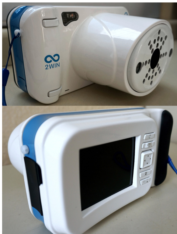
FIGURE 2. 2WIN handheld refractometer
