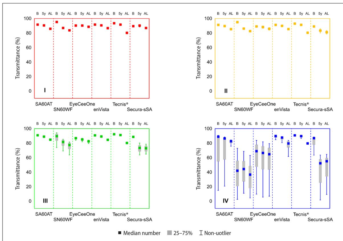
**FIGURE 5.** The transmittance of the tested intraocular lenses (IOLs): initial (denoted as “B”), after 57 days in phosphate-buffered saline (PBS) at 85°C (simulated 5 years in the eyeball, denoted as “5y”), and with the albumin layer deposited after the durability assay (denoted as “AL”). I — red-orange (589–780 nm), II — green-yellow (530–589 nm), blue-green (470–530 nm), violet-blue (380–470 nm) part of the visible light spectrum
