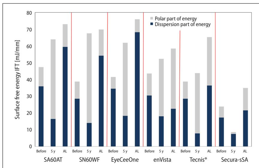
**FIGURE 4.** Changes of surface free energy with polar and dispersive part of the energy for all types of intraocular lenses (IOLs) tested: initial (denoted as “Before”), after 57 days in phosphate-buffered saline (PBS) at 85°C (simulation of 5 years in the eyeball, denoted as “5y”), and with albumin layer deposited after the durability assay (denoted as “AL”)
