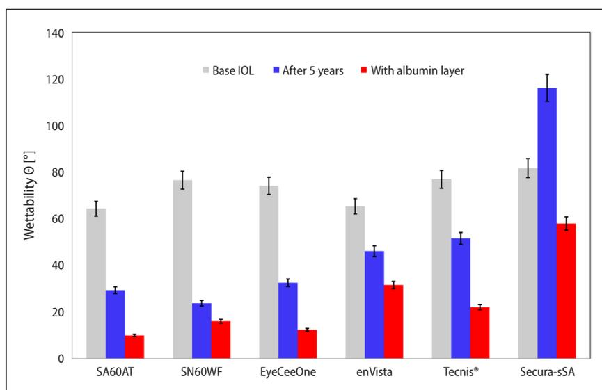
**FIGURE 3.** Wettability of the tested intraocular lenses (IOLs): initial, after 57 days in phosphate-buffered saline (PBS) at 85°C (simulation of 5 years in the eyeball), and with the albumin layer deposited after the durability assay
