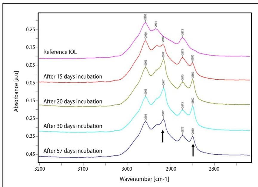
**FIGURE 2.** Attenuated total reflectance Fourier transform infrared spectroscopy (FTIR-ATR) spectra of the initial enVista intraocular lens and after 15, 20, 30, and 57 days in phosphate-buffered saline (PBS) at 85°C corresponding to 96, 128, 192 days
