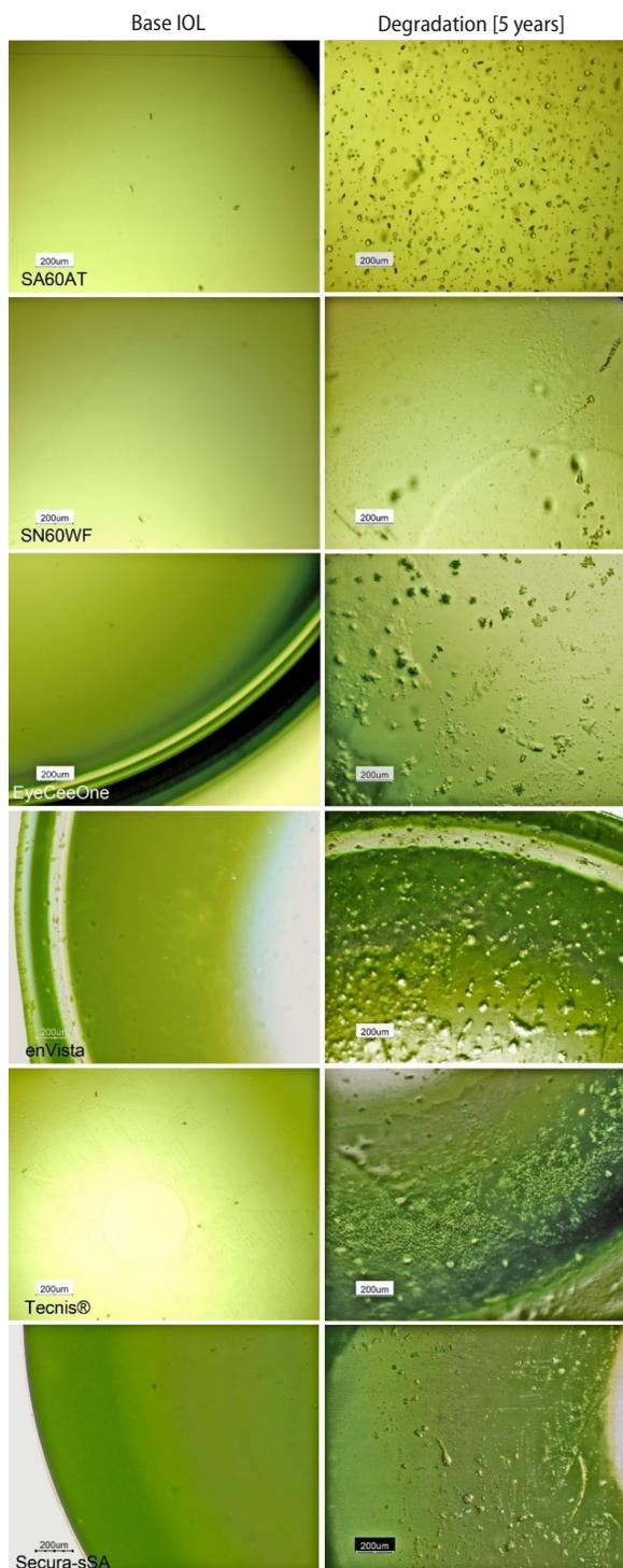
**FIGURE 1.** Representative microscopic images of initial intraocular lenses (IOLs) (base IOL) and IOLs after aging [simulated 5 years of *in vitro* degradation: 57 days/85°C/phosphate-buffered saline (PBS)] with glistening visible on the surface
