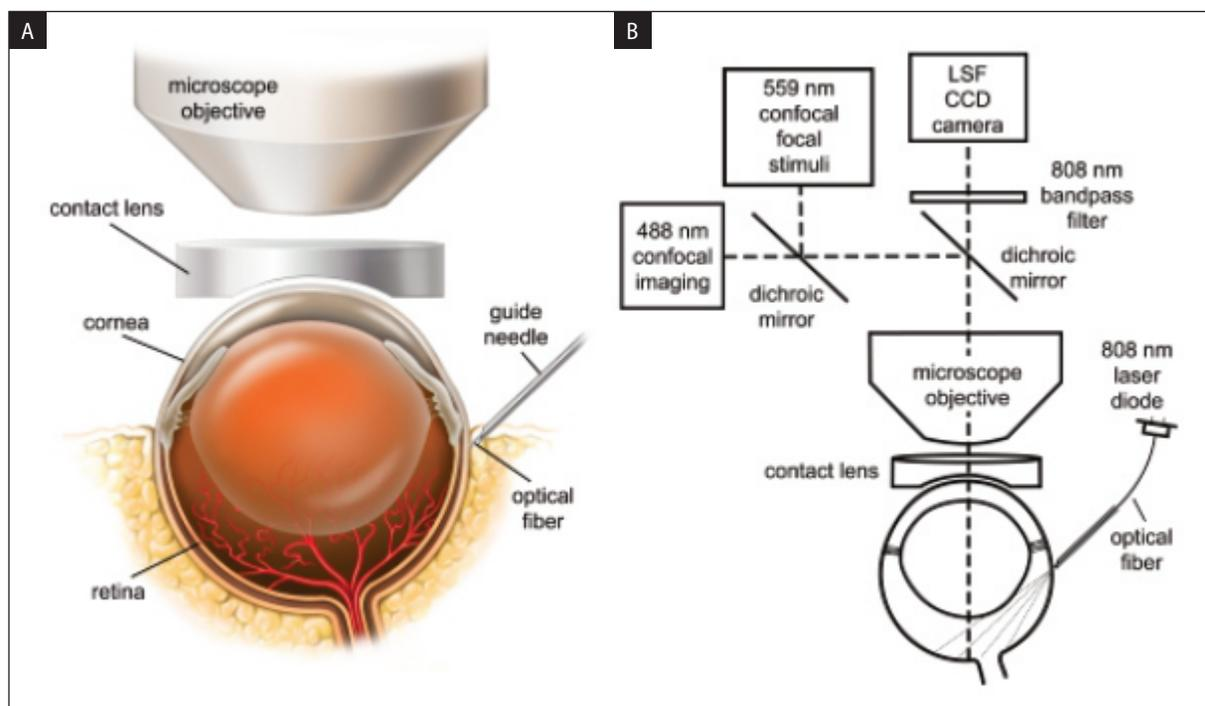
**FIGURE 1.** A schematic representation of the including laser speckle flowmetry (LSF) setup method — the retina is imaged simultaneously through a microscope for LSF and confocal microscopy. Dichroic mirror detects wavelengths for both instruments. 488 nm microscope scans blood vessels, while a 559 nm microscope generates stimulated light. Source: [4], reprinted based on license Creative Commons Attribution 4.0 International
