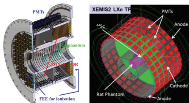
Figure 5. Xemis2: The full three gamma imaging principle
