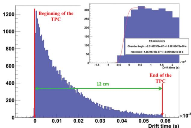
Figure 4. Drift time measurement and drift time resolution
