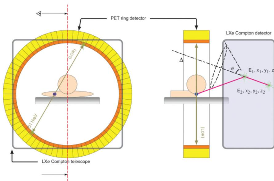
**Figure 1.** Principle of 3  $\gamma$  imaging
