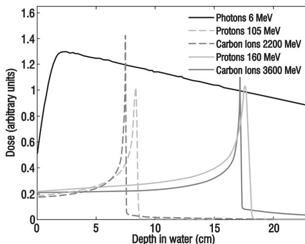
**Figure 1.** Calculated depth-dose deposition in water for monoenergetic photon, proton and carbon ion beams in the energy range of therapeutical relevance. For the photon beam, an additional filtering layer of 2 mm aluminium was included in the calculation prior to the entrance in the water target. Taken from [1]
