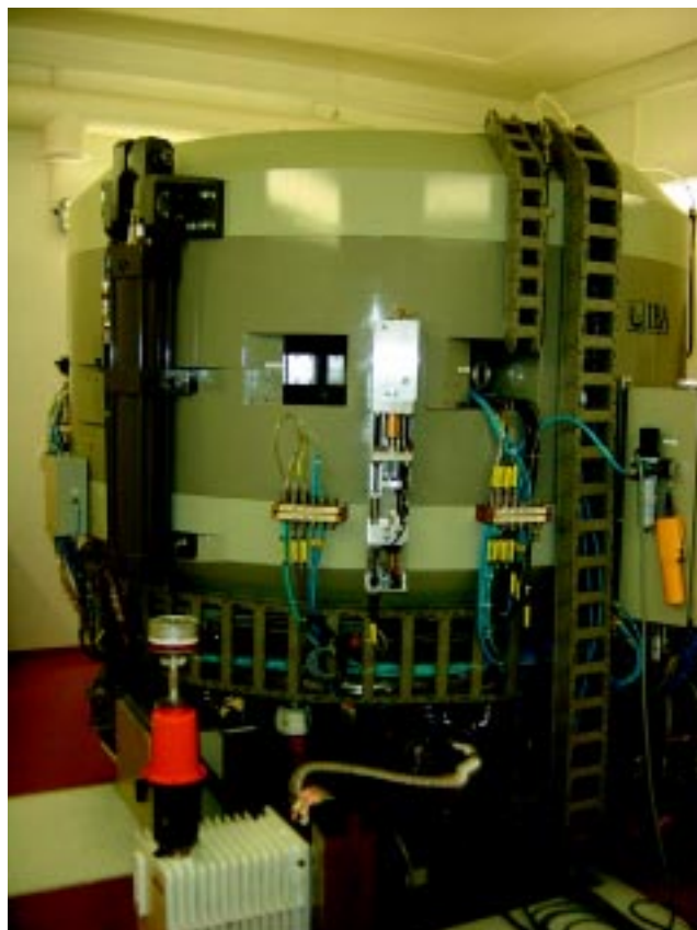
Figure 6. Cyclotron IBA, model Cyclone 18/9.
