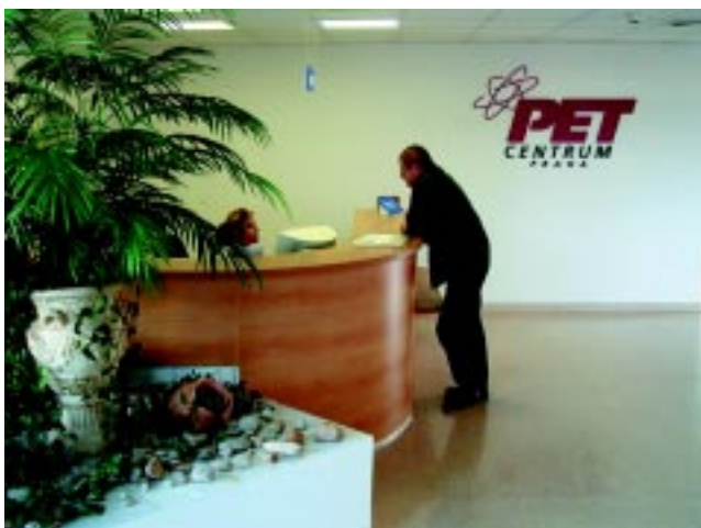
Figure 5. Entrance area. The receptionist is shielded by a concrete-filled counter.
