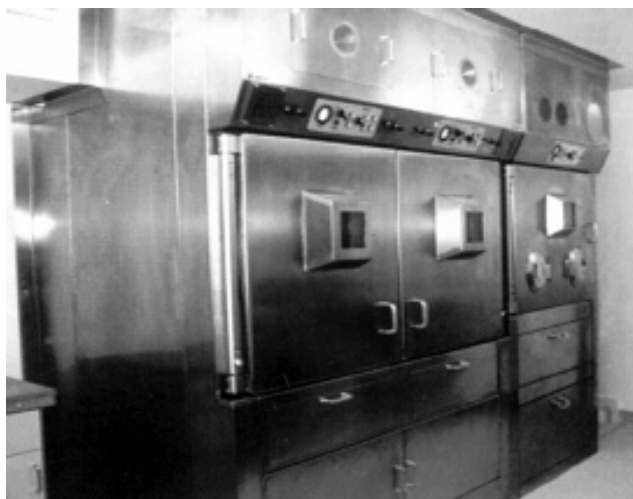
Figure 4. F18-FDG synthesis and dispensing unit.
