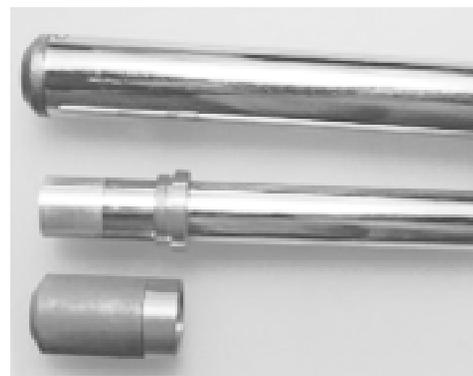
**Figure 4.** The Gamma Ray Prospector's Detector Probes, GRP1 combined with collimator (upper probe) and GPR2 with collimator (lower probe).
