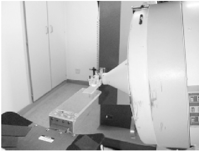
Figure 2. Pinhole-SPECT setup as used in this study employing conventional single headed gamma camera (Siemens Orbiter) equipped with a 2 mm pinhole aperture.
