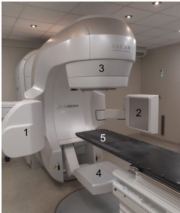
Figure 1. TrueBeam therapy accelerator (Varian Medical Systems, Palo Alto, USA) with: 1 – kV lamp; 2 – kV radiation detector; 3 – accelerator head; 4 – MV radiation detector (EPID); 5 – therapeutic table
