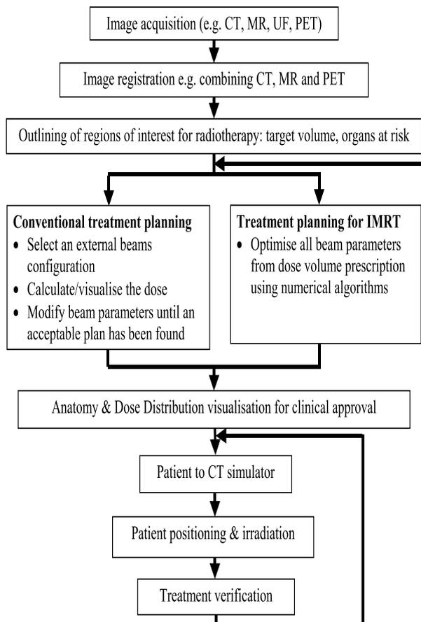
**Figure 3.** Flow chart of the radiotherapy treatment planning process from image acquisition to treatment verification
