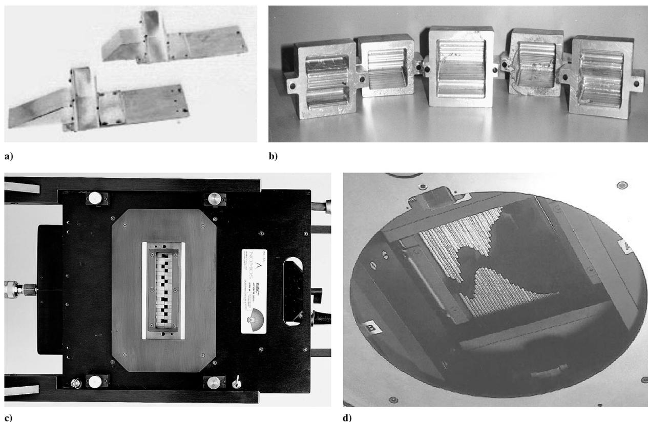
**Figure 2.** Beam modulation devices. [a] Wedge compensators. [b] Compensator designed for an individual patient. [c] MiMic compensator: courtesy Nomos Corporation, USA. [d] Multileaf collimator: courtesy Elekta Oncology Systems, UK
