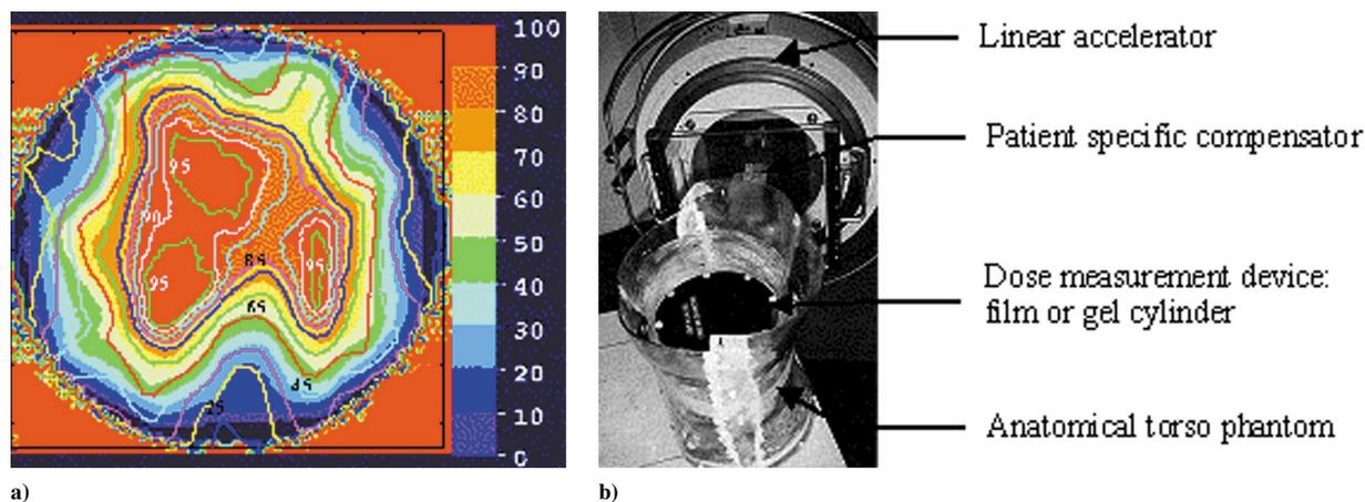
**Figure 4.** [a] IMRT isodose distribution obtained with film dosimetry overlaid on the MR image of the bis-acrylamide-nitrogen and gelatine (bang) gel also used to measure the radiation dose delivered to the PTV and adjacent tissues. [b] Compensator + linear accelerator based IMRT set-up used for the experimental measurements
