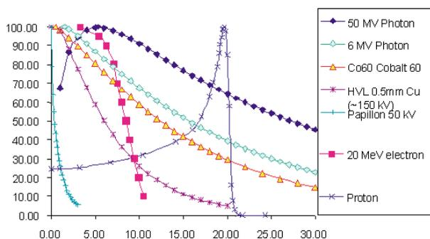
**Figure 1.** Comparison of central axis percentage depth doses for photons, electrons and protons
