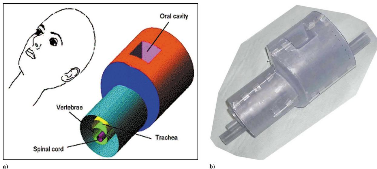
Figure 5. [a] Schematic of the head and neck phantom. [b] Photograph of the phantom
