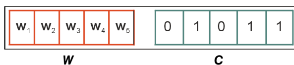
Figure 16. Encoding of the chromosomes for an imaginary treatment case with five possible catheters out of which three are used
