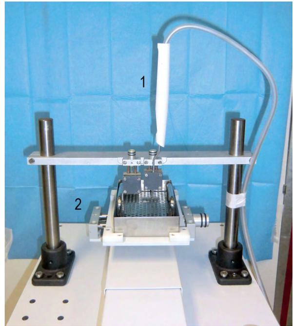
**Figure 1.** Computer-controlled linear device (Software Servomanager 6.4.1, Parker Automation; Erbe Elektromedizin Company) for application of waterjet dissection. Bayonet-shaped waterjet applicator (1) is placed above platform for animals with movement control (2)
