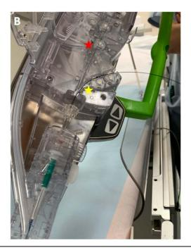
**Figure S1.** The CorPath GRX (Corindus Vascular systems) consists of two separate components: the robotic arm and device cassette shown here and the control console (*Figure S2*). Following coronary cannulation the guiding catheter is (**A**) connected to the robotic cassette (green star) and fixed in a stable position. The device cassette is then used to insert the required wires (red star) and devices (yellow star) which will be controlled by the operator on the separate console
