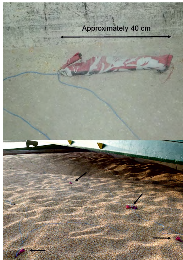
Figure 2. Example of fumigation by aluminium phosphide on board a bulk ship. Top panel: A typical fabric retainer or “sock” containing solid aluminium phosphide (AIP). Bottom panel: Distribution of aluminium phosphide in “socks” (indicated by black arrows) on top of a grain cargo on a bulk ship. The photographs are from the bulk ship Arklow Meadow at port of Warrenpoint, Northern Ireland, December 2012 and are reproduced with permission from Marine Accident Investigation Branch (MAIB), Southampton, United Kingdom
