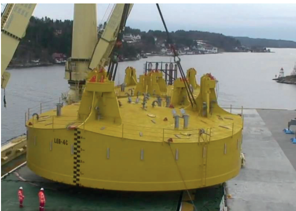
Figure 2. Spud can removed for maintenance
