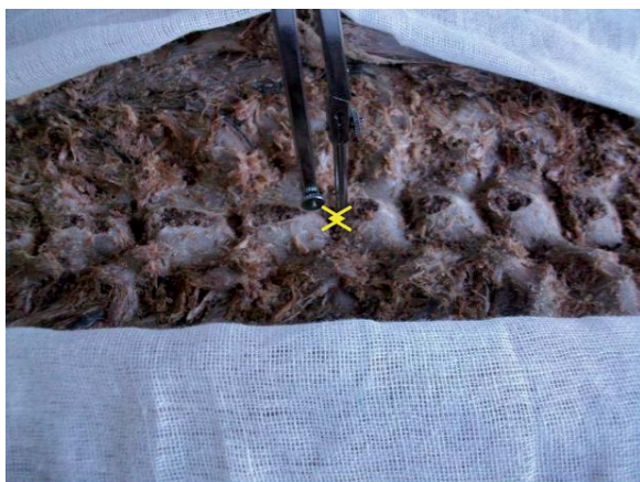
Figure 5. The height of the centre region of lamina space measured with compasses.
