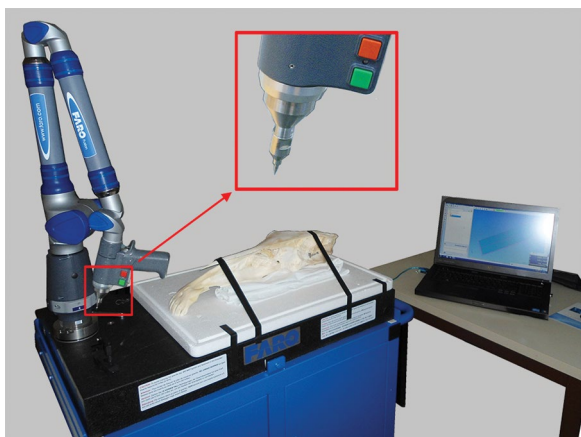
Figure 3. The FaroArm Fusion (FARO Europe®, Stuttgart, Germany) and the experiment setup, with the right half of an equine skull placed and fixed (black fixation tape) on a polystyrene mat in a standardised position. Inset in the red box: magnified image of the tip of the measurement arm.
