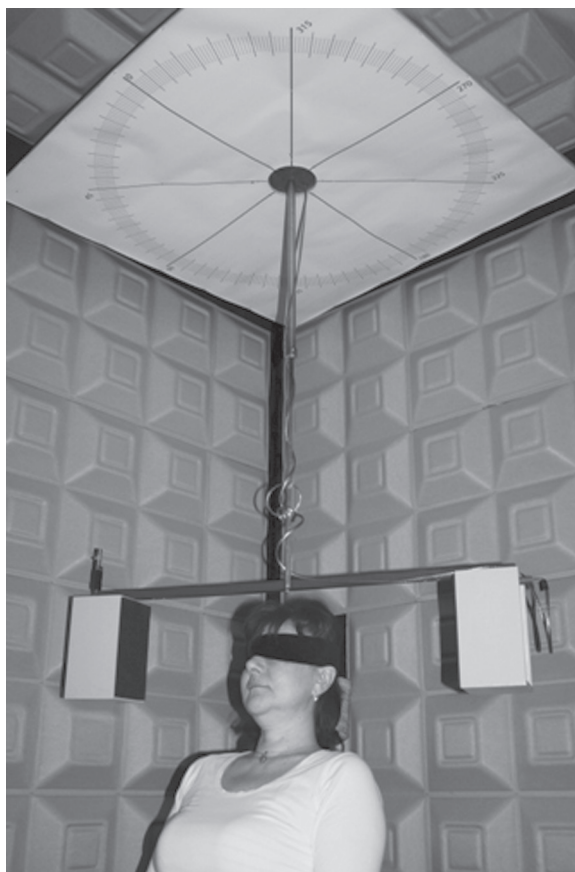
Figure 2. Horizontal minimum audible angle (HMAA) study in a 51-year-old woman. View from sound-proof booth.
