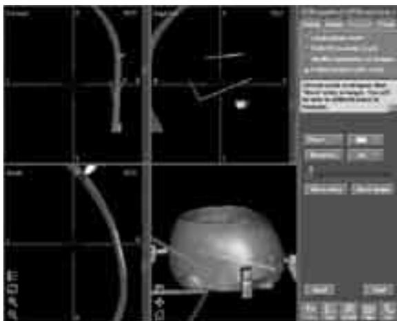
**Figure 1.** A screenshot of a navigation system during the measurements of a phantom approach. On the right upper view the measured pentagon is visible. On the right lower view the three-dimensional reconstruction of the resin phantom is visualised.
