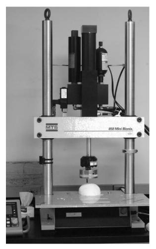
Figure 1. Hydraulic press set up as used in our study.
