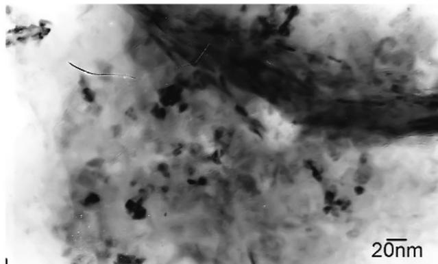
**Fig. 1.** The Transmission Electron Microscope (TEM) photograph for NiO powder. (original magnification  $\times 108\,000$ ).
