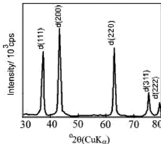
**Fig. 2.** The X-ray diffraction patterns for NiO powder.
