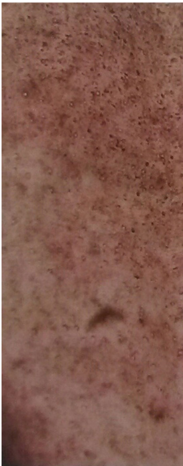
Figure 1. Photo image under microscope of the perfluorocarbons (PFC) nanobubble – magnetic nanoparticle conjugate emulsion
