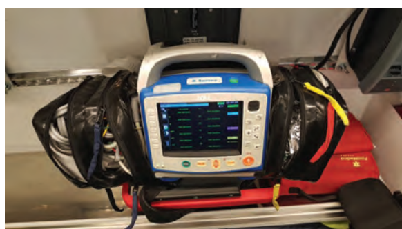
FIGURE 2. ZOLL X series defibrillator equipped with "S" assembly, no. W04-51
