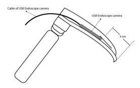
FIGURE 2. Schematic illustration of USB-L
